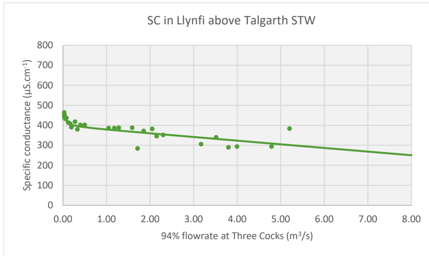
Figure 3: discharge dependency of electrical conductivity in the Llynfi above Talgarth STW
