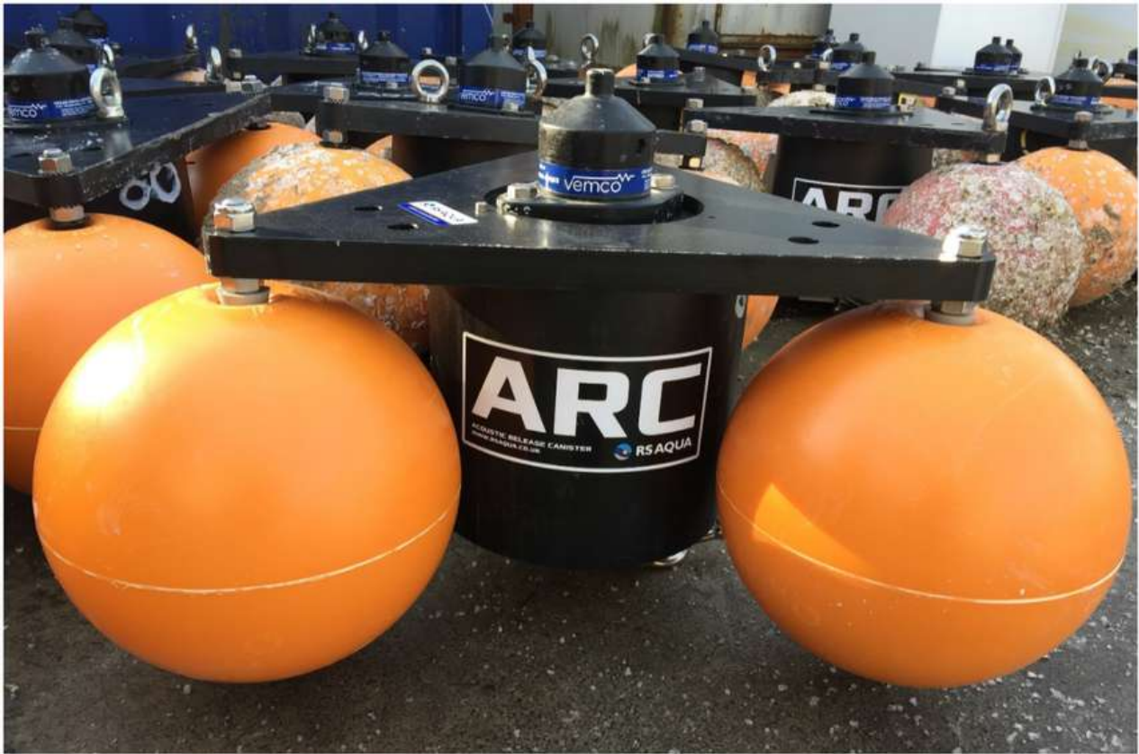
Figure 1: ARC systems with Vemco VR2AR receivers being prepared for deployment. Photo credit Rob Main, Marine Scotland.
