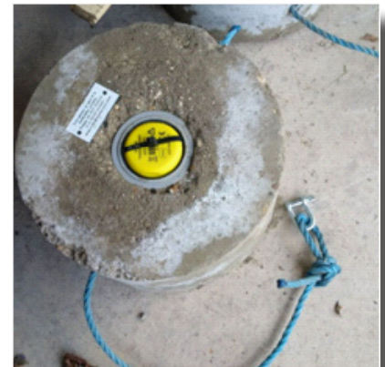
Data logger [yellow] mounted ready to be immersed
